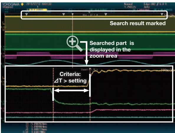
Waveform search using "State width"
