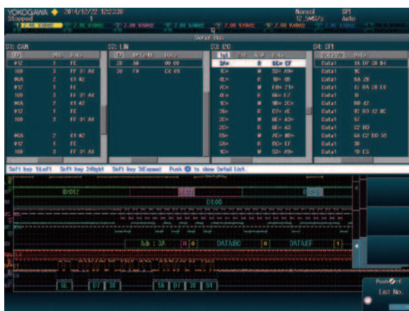
Four bus decode and list display
